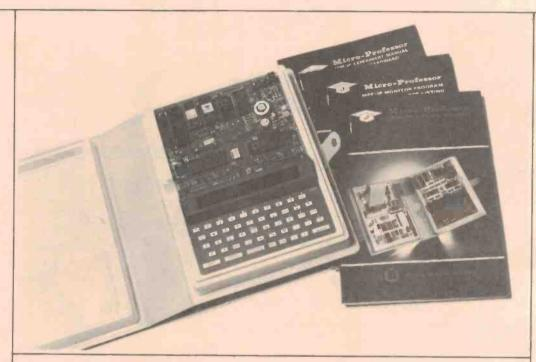
The MPF-1P Microprofessor. This is based on the Z-80 CPU, operates at 1.79 MHz and has on-board 4K RAM and 8K ROM. Other features are a 49-keay keyboard, built-in speaker, interface for program storage/reading to and from cassette, 20-digit, 14-segment alphanumerical green tube display, 48 input/output lines, battery backup for the RAM contents, buss-expandable Z80 architecture and three user manuals.
