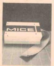
The Mice emulator is controlled via an RS232C compatible interface, and all software necessary to operate it is contained in EPROMs within the module.
