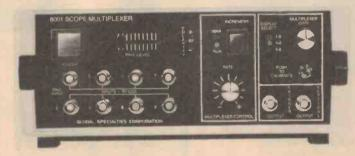
±5 V (10 V peak-to-peak) with a frequency response which is flat to 12 MHz and 3dB down at 20 MHz; input impedance is 1M, G.S.C. claim.
