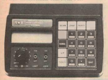
The three reception modes are: narrowband FM (NBFM) of ±7.5 kHz deviation, wideband FM (WBFM) of ±50 kHz deviation, and AM for modulation bandwidths to 50 kHz.
